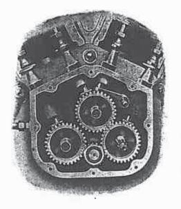
Arrangement of Timing Gear 7.99 h.p. A.J.S. LILUSTRATION E.
