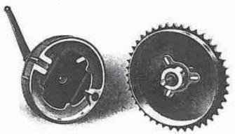
The A.J.S. Internal Expanding Rear Brake. The Expanding Shoes are shown detached from the Drum. ILLUSTRATION S.
