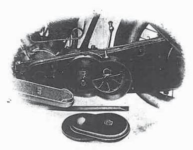
A.J.S. Chain Case with Front Cover removed, exposing Clutch and Foot Starter. The hinged Covers for Chain Inspection are also shown.
