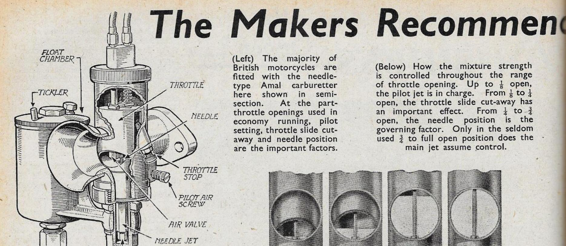
(Left) The majority of British motorcycles are fitted with the needletype Amal carburetter here shown in semisection. At the partthrottle openings used in economy running, pilot setting, throttle slide cutaway and needle position are the important factors.
