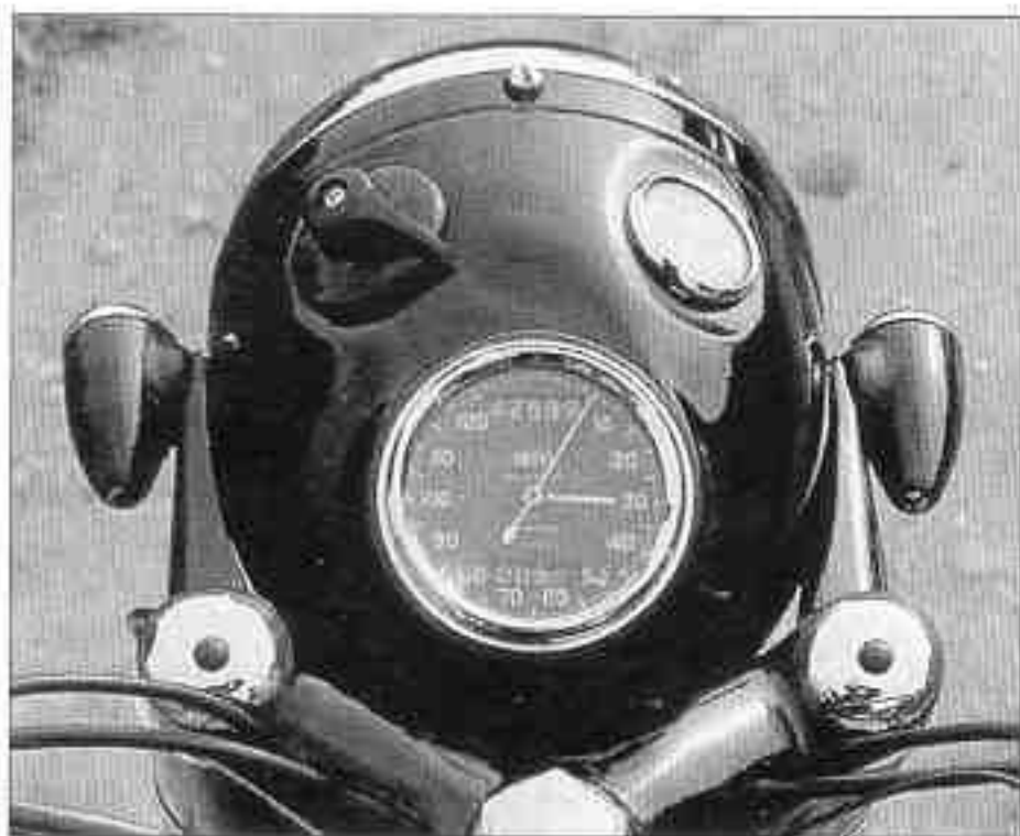
Twin parking lights add that Flash Gordon touch to the Model 30's headlamp assembly
