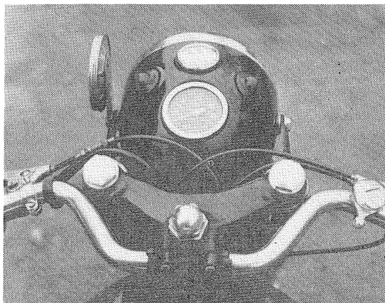
Lights are controlled by the lefthand switch in the headlamp, ignition by the righthand one (which has an emergency starting position). The ammeter needle, partially shrouded by a plate in the dial face, can be seen well enough by the rider
