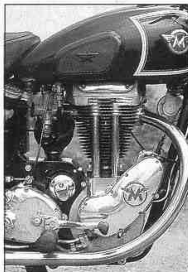
Magneto-equipped engine is the best-looking, but Burman B52 gearbox demands slow-motion changes
