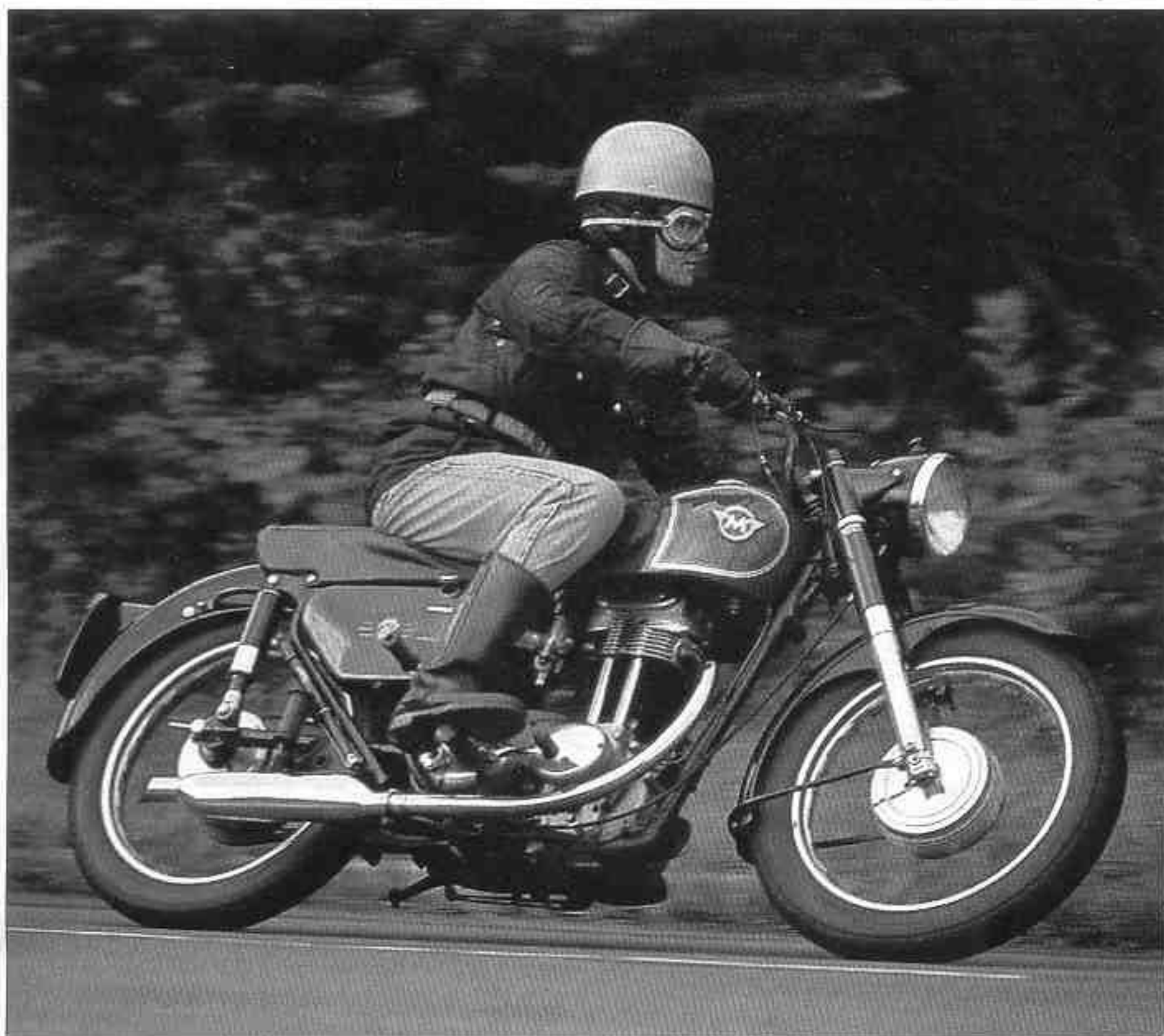
1958 G3LS Single downtube chassis can be swung confidently through bends
