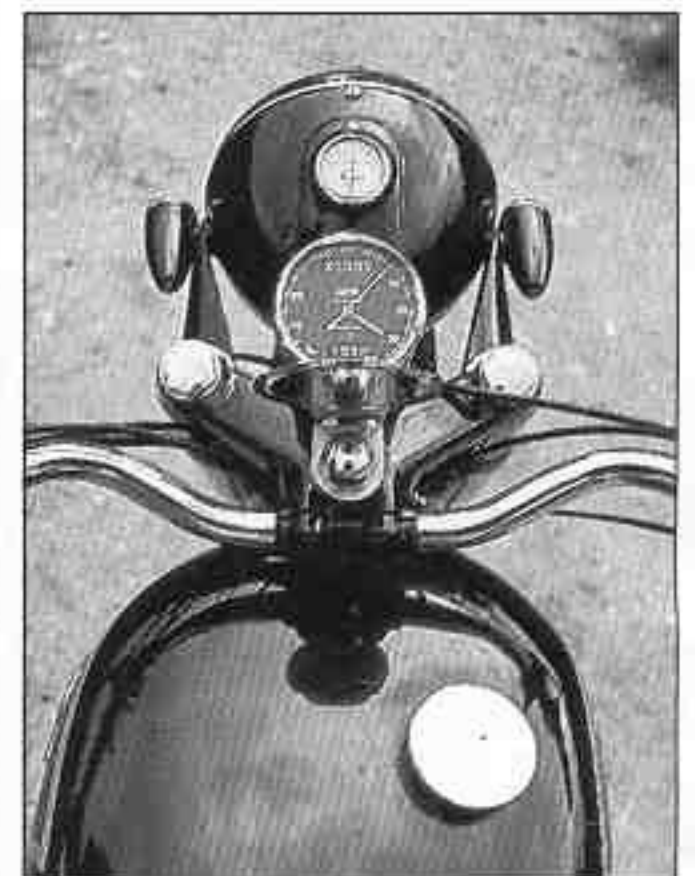
Twin parking lights mounted either side of headlamp are more stylish than practical. Speedo is Smiths Chronometric
