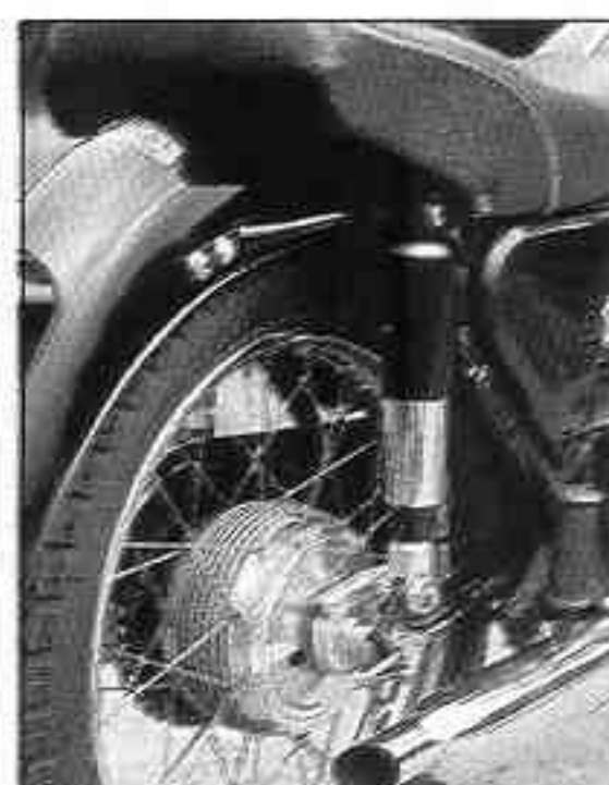
Girling rear units have AMC's lower clevis mounts. Rear mudguard hinders wheel removal
