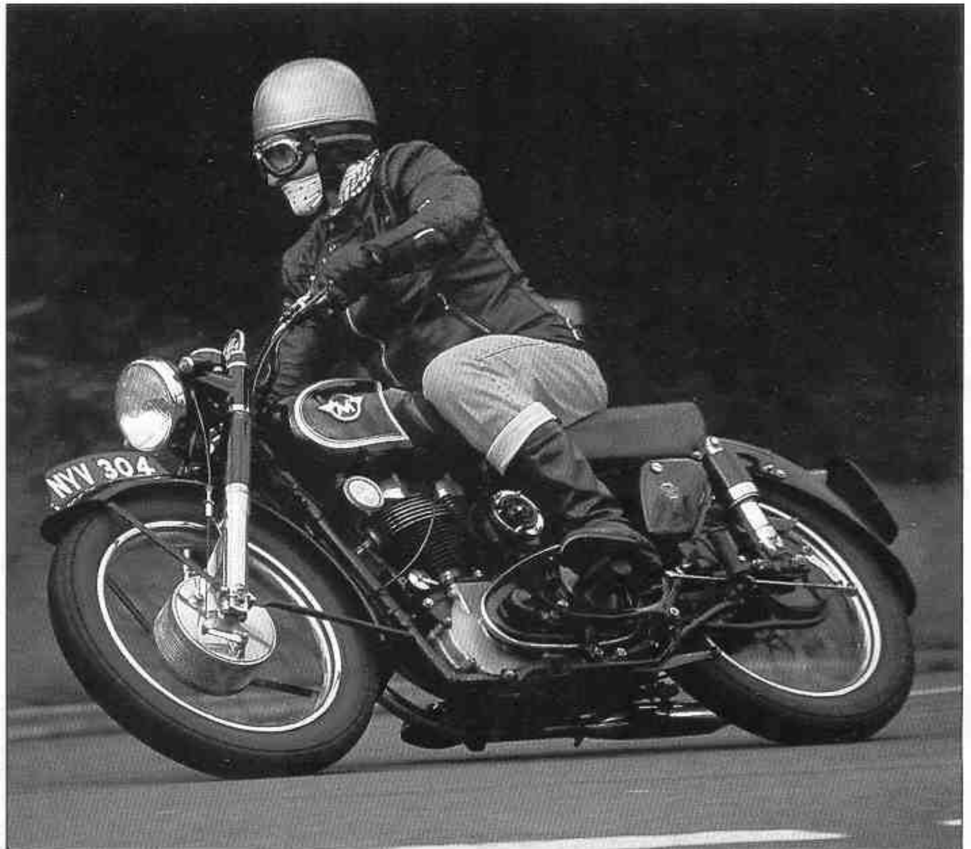
1954 G3LS Suspension is softest on the earlier model with front fork dive under braking
