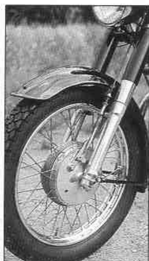
Full-width 7in front brake is best described as adequate rather than exceptional
