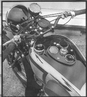
The 1937 Model 72 has fully adjustable handlebar links for complete comfort.
