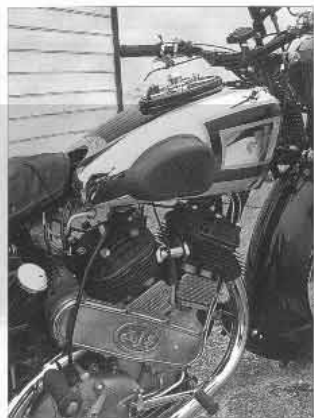
Improved cylinder head finning and positive valve gear lubrication for 1937.
