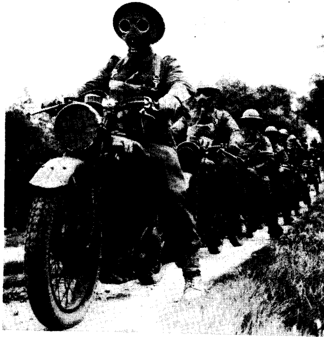
The famous heritage of the AMC singles is well illustrated by this 1941 shot of WD three-fifty Matchless in a wartime inter-services exercise. Note the girder front fork. In that year the Teledraulic fork made its appearance; it was the first of the modern generation of telescopic front forks
