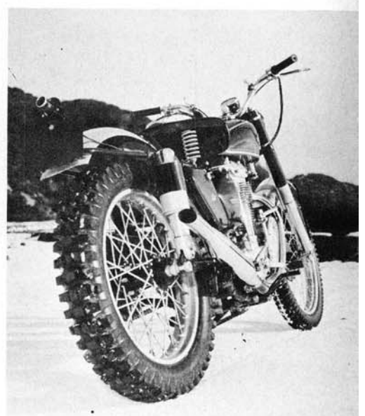
Rear wheel is practically geared to road for slugging. Fender braces are mounted outside to help keep inside of fender from loading up in mud
