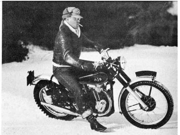
High Scrambles seat position makes it easy to uncoil a leg and stab at the ground when cornering on a slick surface. Rear Dunlop Trials tire held well in snow. Rear shock has compressed almost an inch during turn
