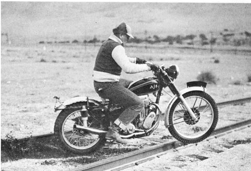
Running between railroad tracks at 5 mph it was possible to turn sharply and ride over and out of the rails without pause or footing. Contributing factors here were bike's short turning radius and high frame clearance. Note contoured exhaust system is out of the way
