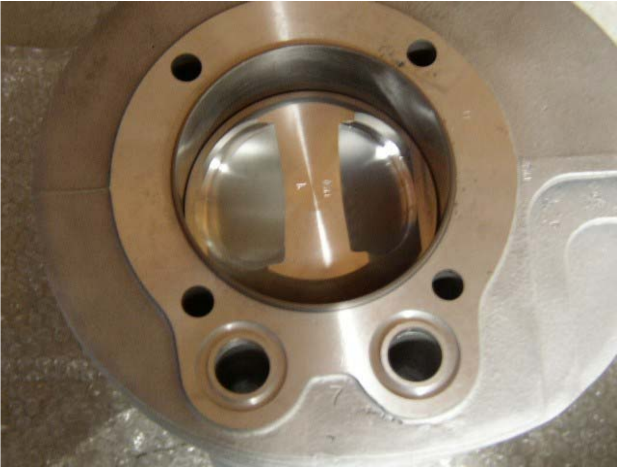
Omega piston and new liner
