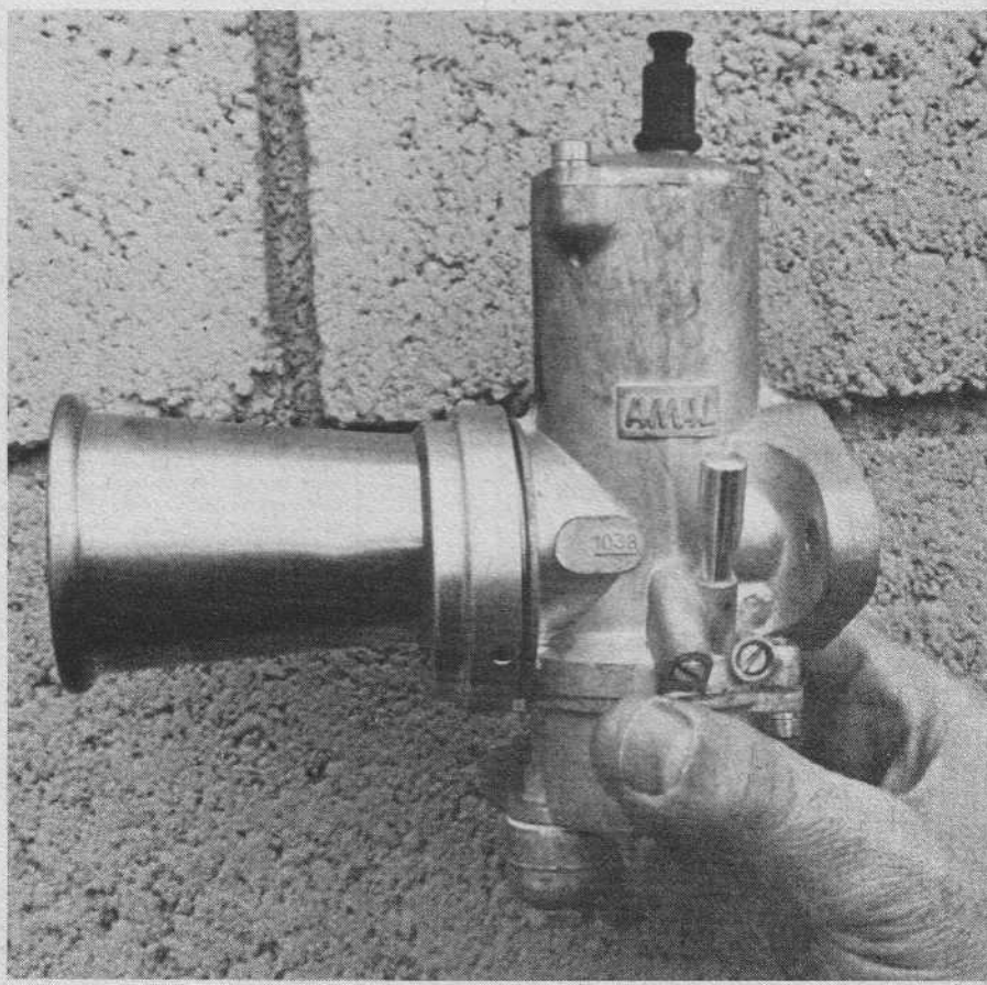
Burak-Bye offers this racing bell as an accessory for the Mark II as well as the Concentric.
