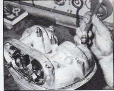
8a With the engine on a bench, remove nine bolts holding rocker box to cylinder head . . .
