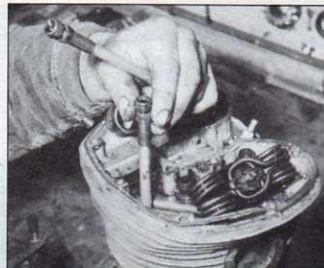
10 Lift out pushrods and label them IN and EX. Examine cups for damage.
