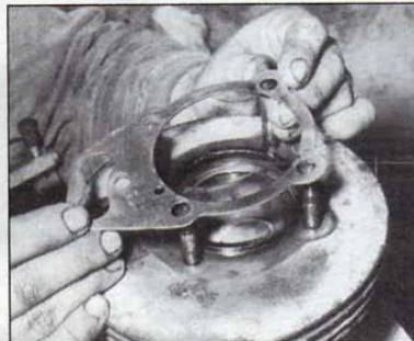
11a Lift the head and examine the gasket.
