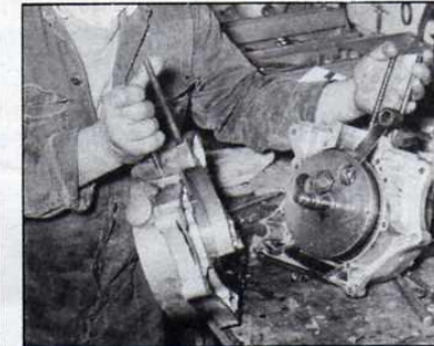
24 Undo crankcase bolts and heat cases. Halves will then separate leaving ball bearing in case. Renew mains and big-end as necessary.
