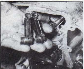
19 Remove cam followers, noting spacers. Smaller of the two goes in the middle.
