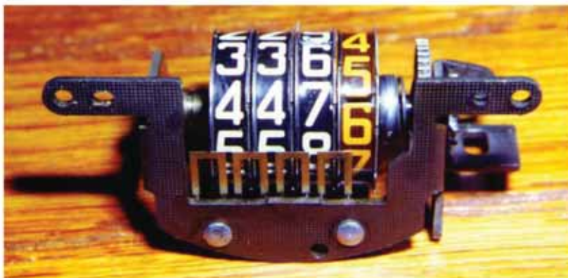
Figure 11. An "early" trip odometer incorporating wheels identical to the main odometer. The trip odometer is mounted on its own sub-frame. The metal fingers are shown holding the wheels. It is clear how each wheel can release the finger restraining the wheel to the left.
