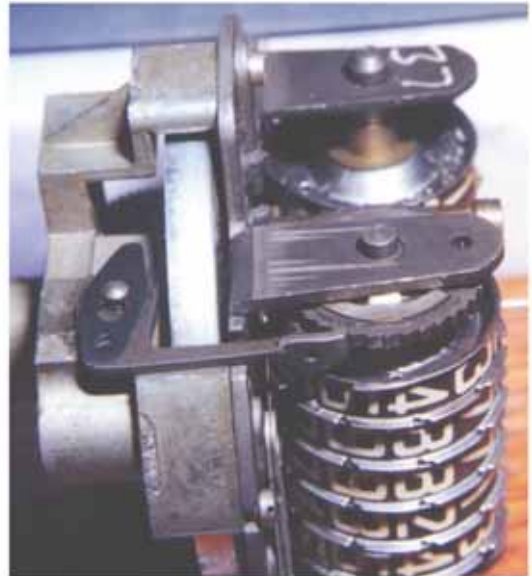
Figure 19. A view of the left of an old-style speedometer. Note the all-metal construction. The shiny thin metal against the left side of the odometer drive gear is the combination retaining washer/ratcheting lock. The number "37" written (by the manufacturer) on the frame is the number of teeth on the odometer drive gears.
