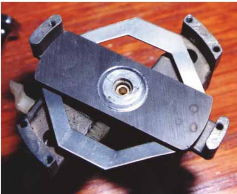
Figure 5. This is a view of the front of the magnet wheel after removal of the odometer wheel frame. In the center is the brass bushing in which the spindle of the pointer rides.
