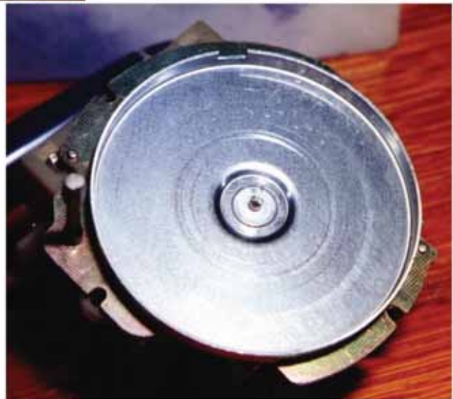
Figure 4. Now the odometer wheel frame has been removed from the magnet wheel frame. This is a view of the underside of the odometer wheel frame with the attached drag cup. In the center of the drag cup is the thin spindle which fits into the bushing in the center of the magnet wheel.
