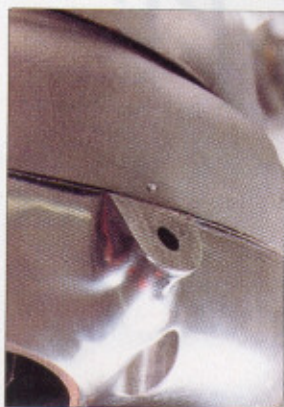
▲ Punch inner cover in line with cable entry before stripdown
