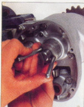
▲ Heat inner cover and then remove clutch lock ring with special tool 01-5800
