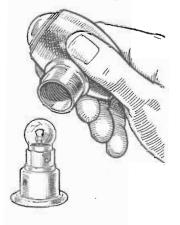
To gain access to the bulb withdraw the securing screw on the lamp stem and then pull the body away from the base. The bulb can then be removed from its holder. Replace the lamp body and secure with the screw.
